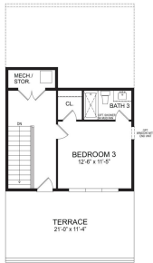
THIRD FLOOR PLAN SHOWN WITH OPT. BEDROOM & BATH @ FRONT AND OPT. END WALL
